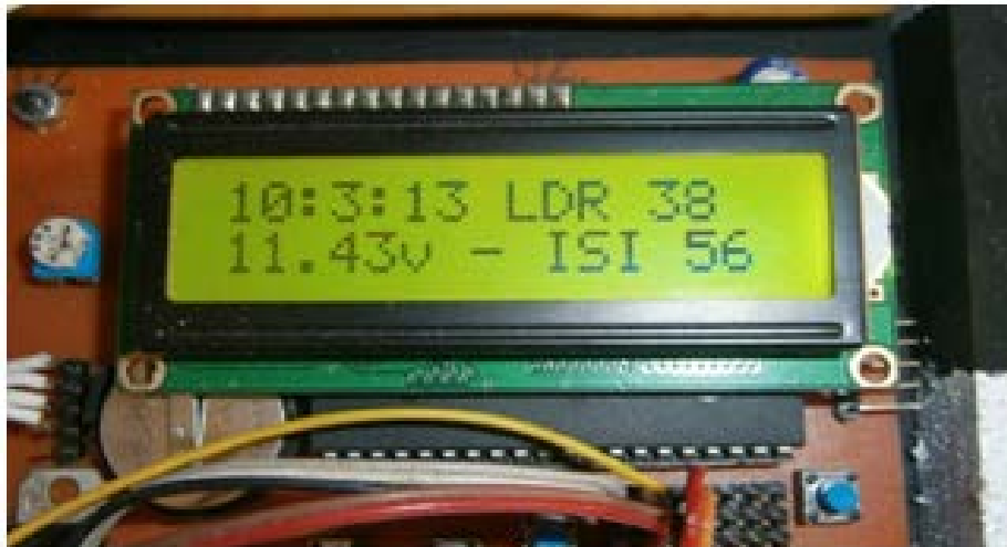
Gambar 8. Hasil Nilai Resistansi Sensor Cahaya
